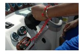
The terms Engine Cut-Off Switch (ECOS) and Engine/Propulsion Cut-Off Devices are used interchangeably to denote a system that disables the propulsion engine when the operator is unexpectedly displaced from the vessel. Most U.S. boat manufacturers have voluntarily installed an ECOS on their boats for decades. It's important to know that, if your boat is equipped with a Cut-Off Switch, the law is that it must be used.
