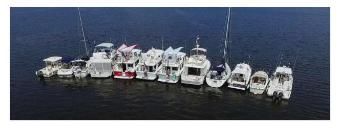
Typical raft ups are straight across, bow to the current or wind. A stern to stern raft up is safer for people moving boat to boat. Sterns will be at about the same height plus the stern or swim platform is flat and designed for traction as visiting across the boats occur. Climbing across slanted bows and over rails is dangerous.
